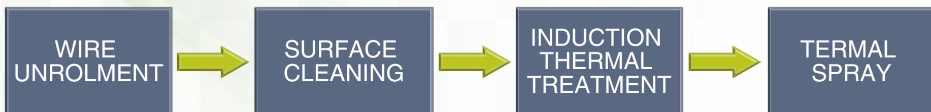
**Fig.4: final realization of thermal spray nozzles**
