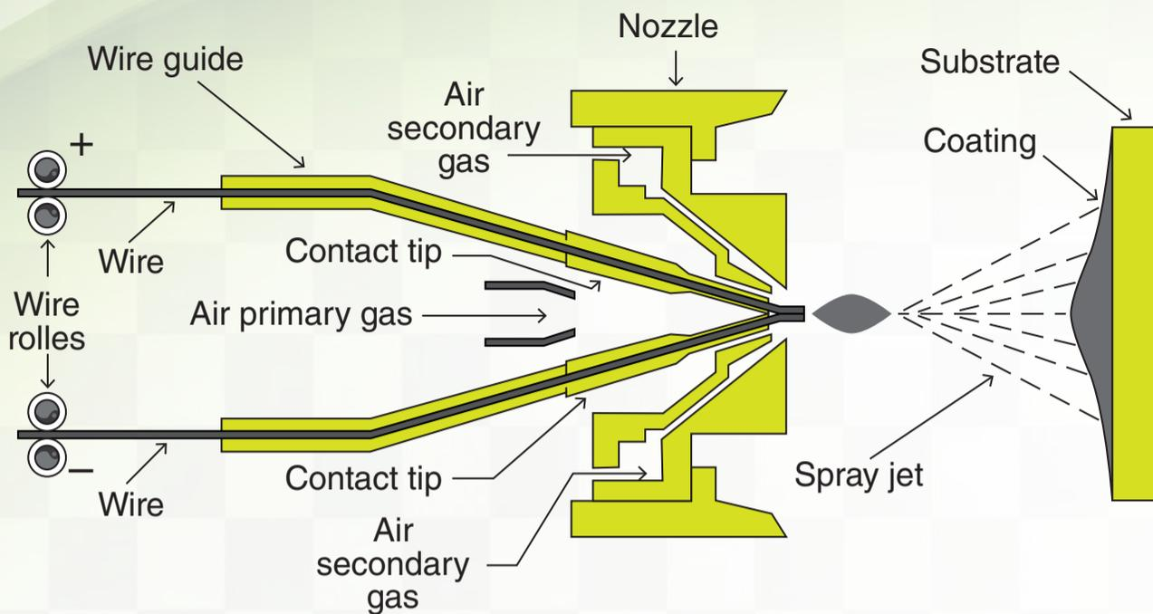
Different thermal deposition techniques are into the category of thermal sprays, which differ only in the way in which thermal energy is applied to the particles to be sprayed and can be divided into three categories:
